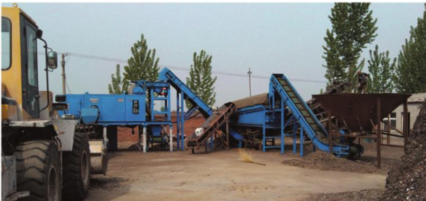
Steel Slag Processing System could deal with waste tailing pollution of steel industry, separate non-ferrous metal, stainless steel, rubber etc from the waste tailings.
